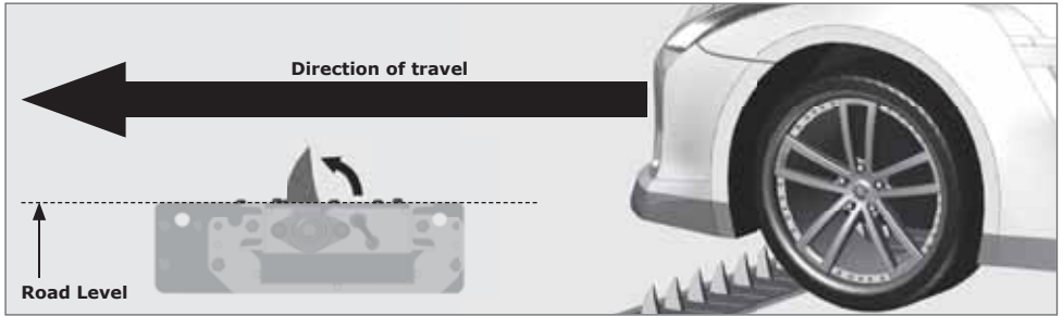
FIGURE 4. SPIKE IMPACT DIRECTION - SIMILAR
