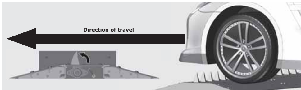
FIGURE 4. SPIKE IMPACT DIRECTION - SIMILAR
