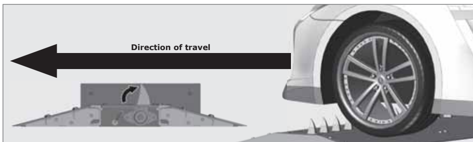
FIGURE 5. SPIKE IMPACT DIRECTION - OPPOSING
